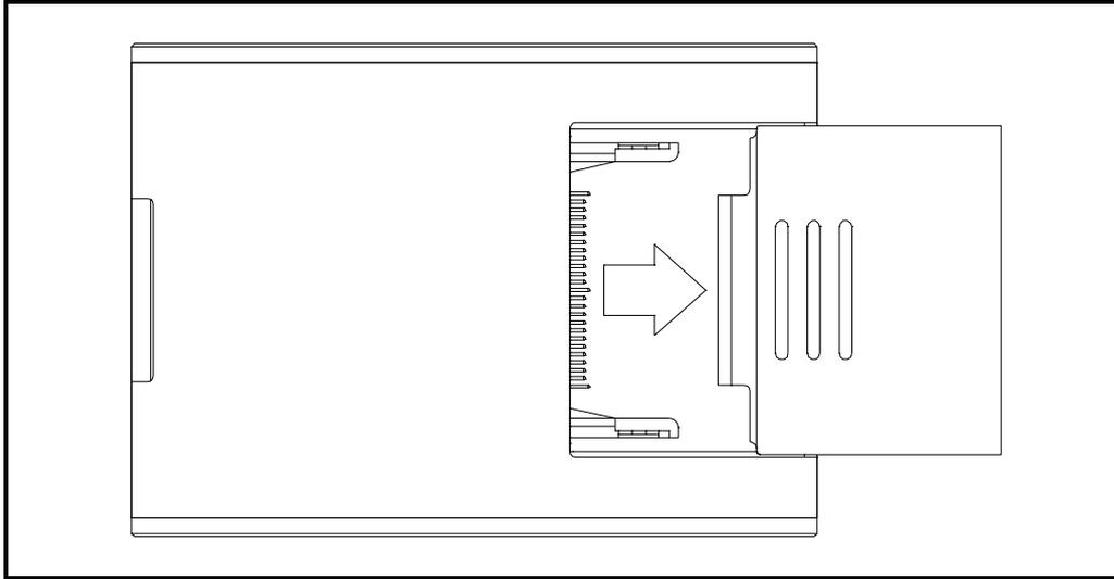
Fig. 1.5 Remove the back cover
