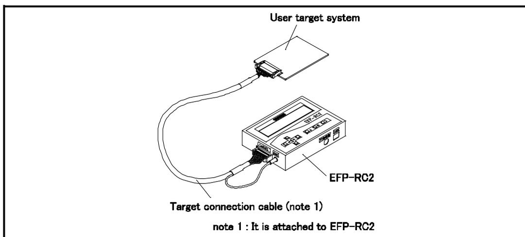
Fig. 1.4 Connection with target system
