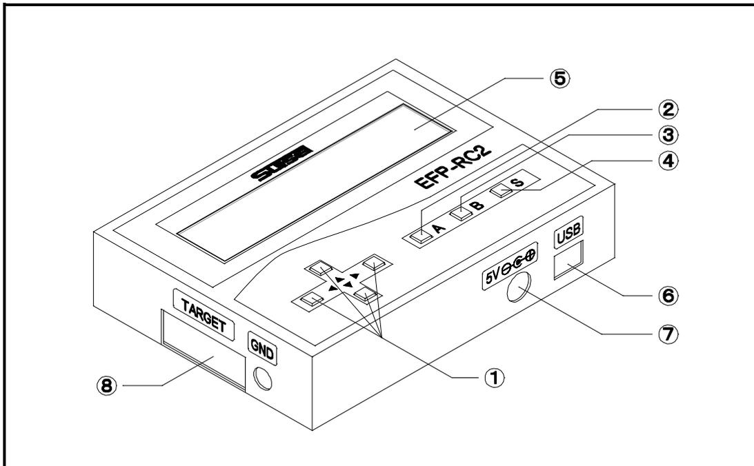
Fig. 1.1 Name of each part of EFP-RC2
