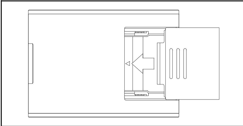
Fig. 1.7 Back cover installation
