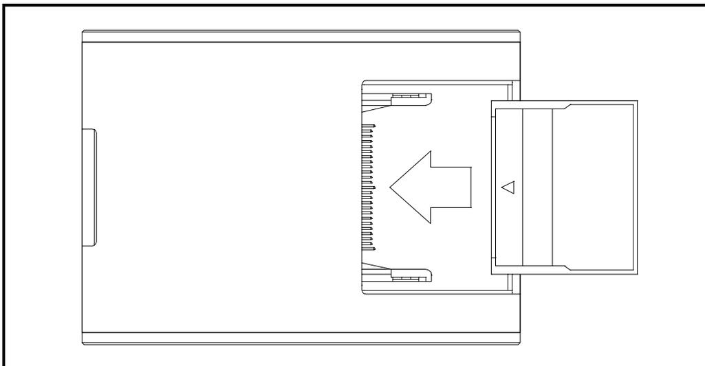
Fig. 1.6 CF card installation
