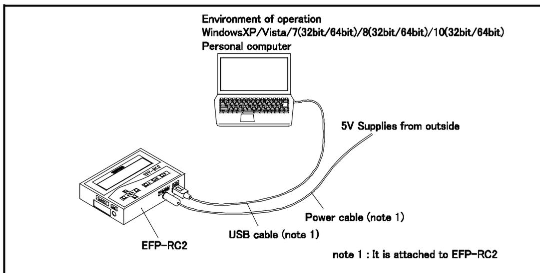
Fig. 1.3 Connection with computer
