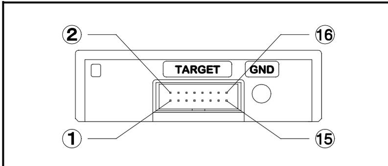
Fig. 1.2 Target connector pin layout
