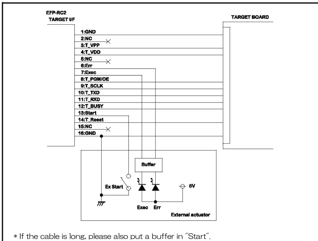
Figure 5.1 Example of external control signal connection
